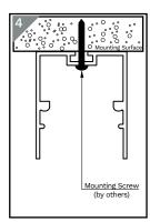
Drill & secure mounting screw to the surface through the luminaire as shown
