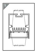
Retrace steps 3 & 2 Make sure all cables are cleared from pinching and geartray is snapped back in
