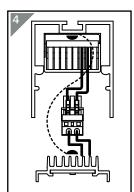
Disconnect connection to service unit. Undo lanyards for geartray upgrade/replacement
