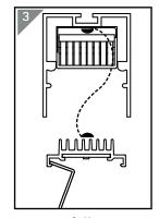
Carefully use Austube Schréder remover tool to remove geartray
